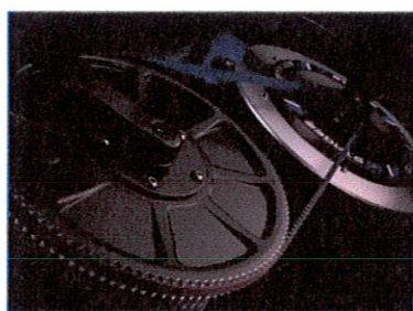
CarbonGlyde™ Featuring Gates® Carbon Drive™ Carbon Fiber Belt
